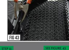
11) Carefully align the t-rex grille so that it sits evenly aligned with the shell and clamp into place.
