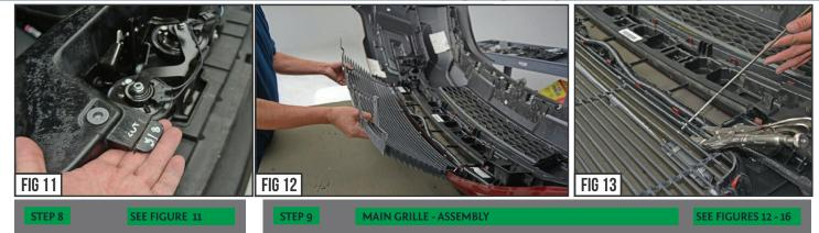
8) Note, that you will need to trim a small plastic tab located on the core support in front of the radiator near the hood latch mechanism.
