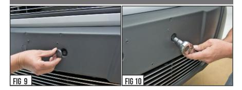
7) Finally, there are (3) clips holding the bumper each side to the wing
