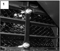
**Step 3.** Making sure that the grille is centered; tighten down all the hardware. Re-place the upper motor cover. Some of the holes on the top plate should line up with holes in the factory motor cover and utilizes the factory clips. *Thanks for purchasing your T-REX grille, 03-26-08*
