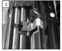
**STEP 2:** Open the hood of the vehicle. Insert the new grille into the factory bumper opening. With the grille centered; place the provided screws from the front side of the grille into the provided J-Hook (2).
