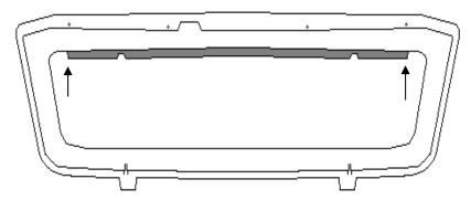
Cut the center cross bars out of the grill shell. Leave a 3"- 4"plastic lip along the top of the opening from corner to corner (note shaded area in the diagram). Make your final cuts as close to the face of the grille as possible. This will allow the billet insert to sit flush to the front of the grille shell. Use a file or sand paper to smooth a straight edge around the opening.
