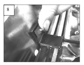
Center the billet grille inserts behind the grille. Bend the brackets on the grille so they sit flat against the grille shell. Make sure the polished billet bars sit in each opening. If they do not align correctly, adjust the brackets.
