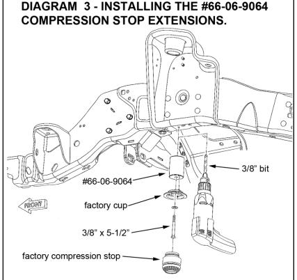
cup is positioned toward the inside of the vehicle as shown in Diagram 3, then tighten the 3/8" bolt (23).
