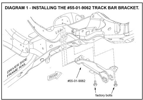
[DIAGRAM 1] Position the Superlift<sup>®</sup> track bar bracket (#55-01-9062) on the frame in the same place as the original and secure using the factory hardware. There are a total of five bolts; three attached to a retaining tab plus two additional bolts. Once all the bolts are started, tighten (136).
