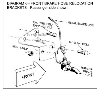
using the factory self-tapping bolt. The rearmost top hole takes the supplied 5/16" x 1" self-tapping bolt. Some vehicles will require this hole to be drilled out to 9/32". Carefully pull down and re-form the metal brake line so the rubber hose assembly will bolt to the "16" bracket. Use the furnished 1/4" x 3/4" bolt / Nyloc nut.
