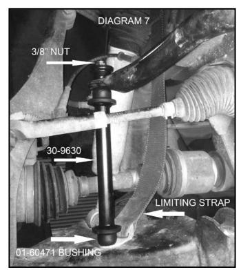
[DIAGRAM 7A] There is a factory hole in the forward lip of the shock tower. Measure down approximately 3/4" from the factory hole, then mark and drill a 15/32" mounting hole for the
