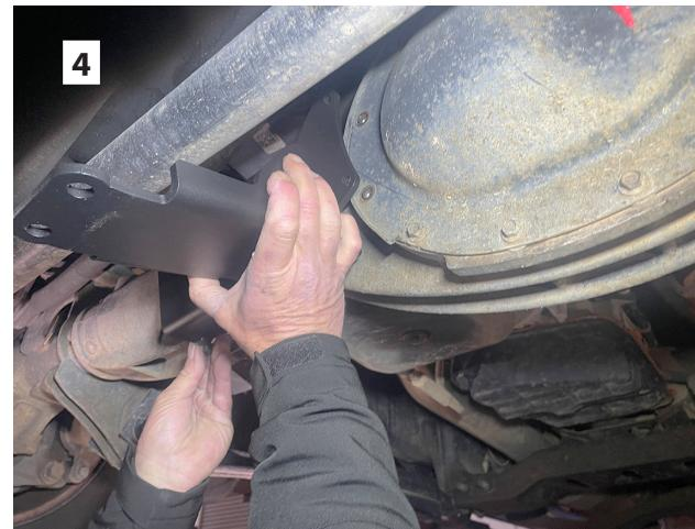
8. [Illustration 5] Place the new differential spacer (55-06-92770) between the center bracket assembly and the differential and secure using supplied 8mm bolts and washers, applying the supplied thread locker to the bolts.
