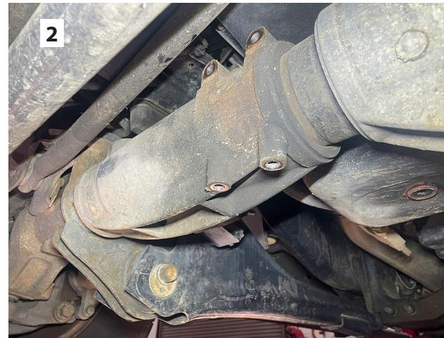
4. [Illustration 3] Remove the factory steering stabilizer mounting bracket from the tie rod.
