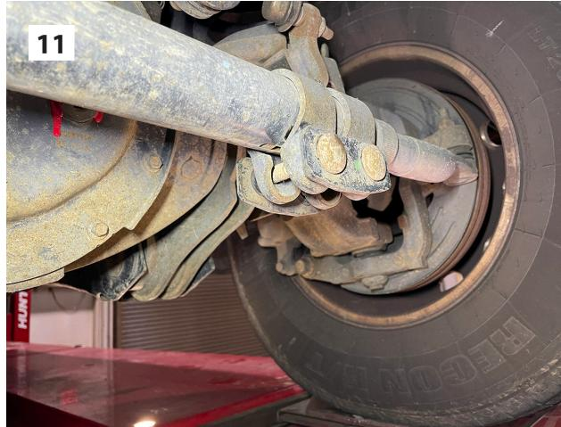
16. [Illustration 12] Secure the new tie rod bracket to the tie rod with supplied 3/8" ubolts and flange nuts.
