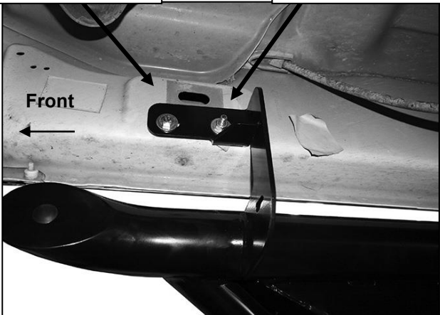
(Fig 9) Passenger/right front 2009-2010 model pictured. IMPORTANT: All models without holes in pinch weld will require drilling 1/4" holes through pinch weld to attach support brackets. Do complete installation of sidebars first, level sidebar before drilling holes for support bracket.
