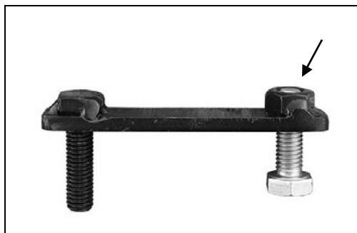
(Fig 4) Thread (1) 8mm Hex Bolt into the nut on the plate. Stop when bolt reaches end of nut as pictured
