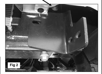
Insert 12mm Spacer Washer between the Mounting Bracket and the frame
