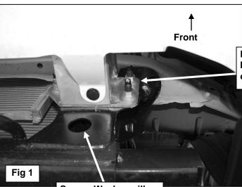
Remove (2) factory hex nuts on outside of frame
