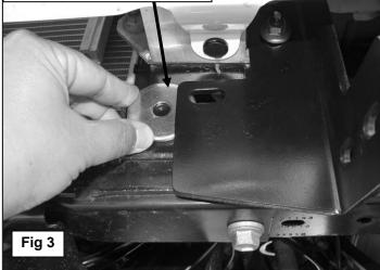
10mm x 20mm Small Flat Washer 10mm Lock Washer 10mm Hex Nut
