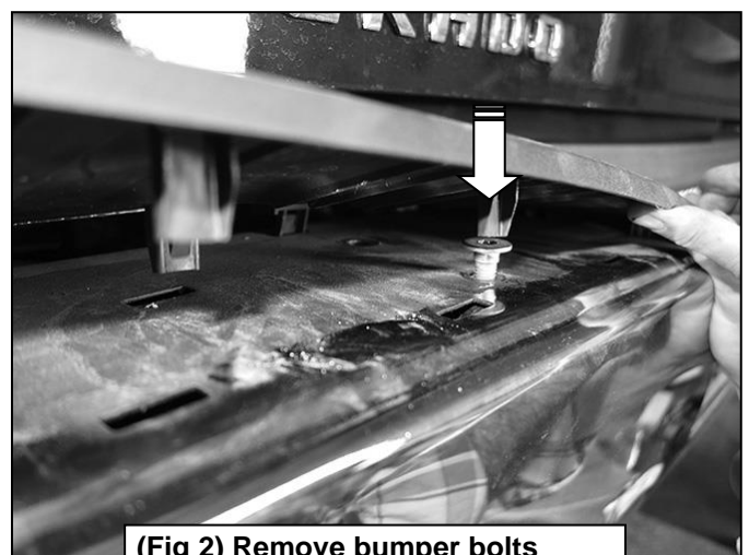
(Fig 2) Remove bumper bolts attaching bumper to inner bracket
