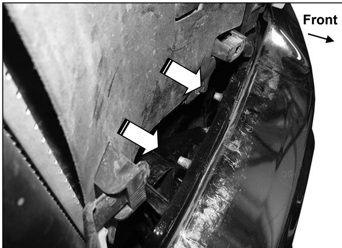
(Fig 3) Remove driver side top bumper hardware
