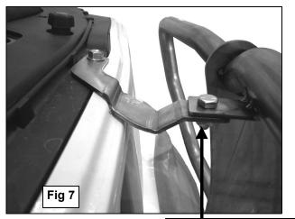
8mm x 20mm Button Head Bolt 8mm Lock Washer 8mm Flat Washer 8mm Hex Nut
