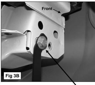
Insert assembly into the factory hole, hold tool handle and assembly up tight against the crossmember and tighten hex bolt until insert is fully expanded into hole, (Figure 4). NOTE: Do not over tighten or a pull out may occur.
