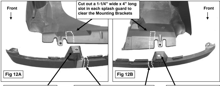
Replace factory hardware for this mounting location with the included: 6mm x 30mm Phillips Screw 6mm Lock Washer 6mm Flat Washer Cut out (2) 3/4" wide slots in the spoiler
