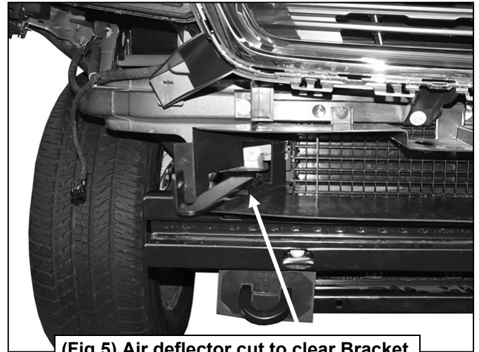
(Fig 5) Air deflector cut to clear Bracket
