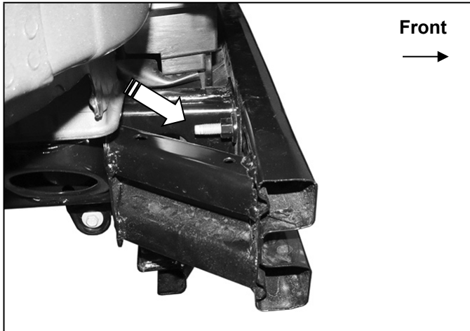
(Fig 4) Top Bracket attaches over factory bolt (arrow). Air deflector removed for instruction purposes
