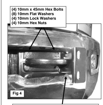
IMPORANT: To prevent damage to the bumper and/or Frame Mounting Brackets, do not allow the Brackets to come in contact, top or bottom, with the steel bumper
