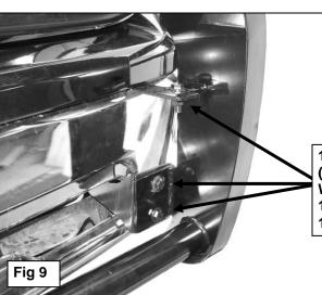
12mm x 35mm Hex Bolt (2) 12mm Large Flat Washers 12mm Lock Washer 12mm Hex Nut
