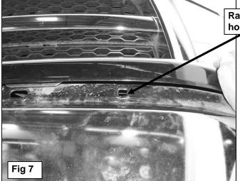
Raise plastic cover to access mounting hole (factory bumper bolt removed)
