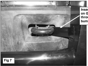
Insert mounting tab on Grille Guard through opening in bumper cover. Bolt mounting tabs on Grille Guard to side of frame channel with factory hardware for tow hook or on models without tow hooks, use:
