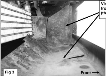
View of rubber air deflector pictured from inside of front bumper (through opening in bumper)
