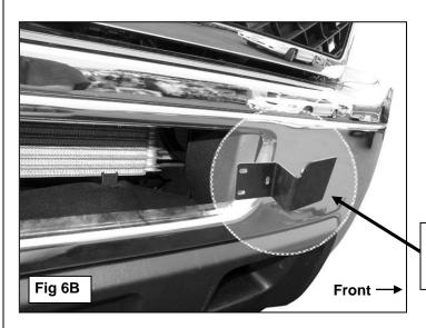
**Driver side Support Bracket illustrated** to show Bracket position inside against the back of the front bumper
