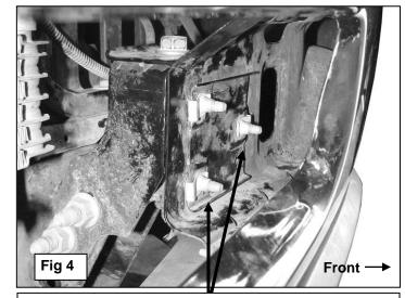
Remove (3) factory hex bolts and cover plate w/clips
