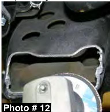
13. The OEM alignment cam brackets (alignment ears) will need to be ground down for the installation of the new Skyjacker cross members. This will have to be done on the front side of both front & rear OEM lower control arm mounts. (See Photo # 14)
