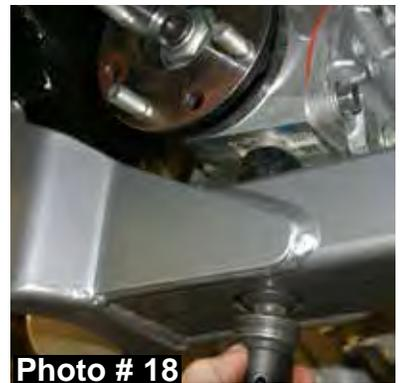
18. Weld in place the new Skyjacker steering stop spacers. Match these new steering stop spacers with the contour of the OEM steering stops. Weld in place by placing a weld across the top & bottom of the supplied spacers. (See Photo # 22)
