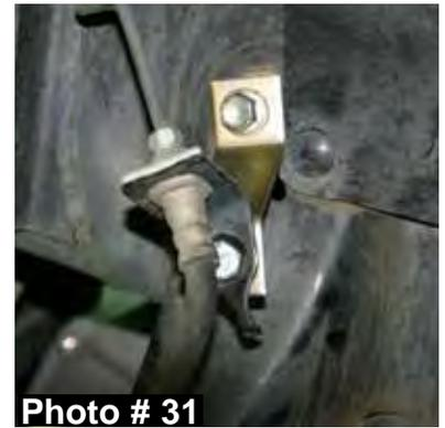
30. To install the OEM outer tie rod ends to the new Skyjacker steering knuckles, the OEM outer tie rod ends will need to be swapped from driver to passenger & passenger to driver side. Attach the OEM outer tie rod ends to the new Skyjacker steering knuckles using the OEM hardware. Reinstall the OEM brake rotors, brake calipers, & etc.
