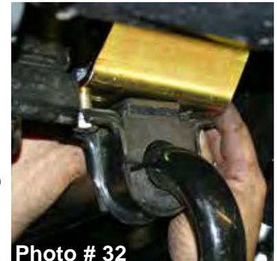
32. Install the new Skyjacker sway bar end links with the pivoting end at the OEM sway bar. **Note:** The new sway bar end links are side specific for passenger & driver side. (See Photo # 33)
