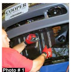
Note: A special PULLER TOOL is required for the safe removal / installation of the torsion bars. This special puller can be purchased from a GM Dealer (Tool # J36202) or from Kent Moore Tool Group, Roseville, MI (800) 345-2233 or (313) 774-9500 (Part # J-22517-C).
