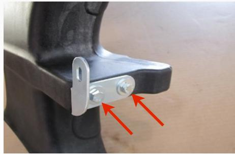
11. Chevy Models Only! Attach the Chevy Bracket (G) to the Scoop (A) using two 1/4"-20x1/2" Hex Screws (D) and 1/4" Washers (E). Then install the Clip Nut (B) onto the bracket.
