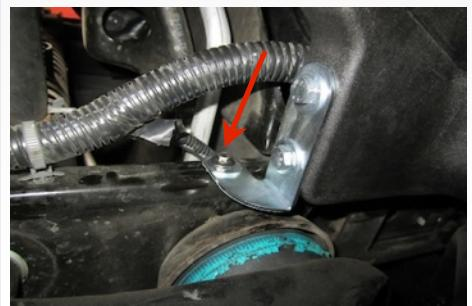
15. Reattach the fender liner to scoop using two 1/4"-20x1/2" Hex Screws (D) and 1/4" Washers (E). Chevy models will use one 1/4-20x1.0" Hex Screw (C) securing the fender liner to the Chevy Bracket (G).
