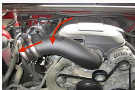
19. Reconnect the MAF sensor wiring harness (and Pressure Sensor if equipped).
