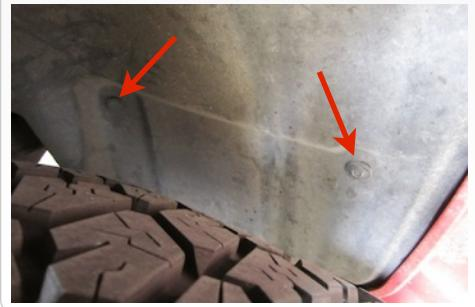
7. Looking through the bottom of the air box, remove the panel pin mounting the plate between the wheel liner and front support.
