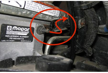
15. Slide the OE t-bolt clamp down the intercooler tube. Push the silicone end of the elbow assembly down over the intercooler tube. Then rotate the elbow assembly over the studs on the heater grid.
