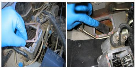
7. Place the supplied Graphite Gasket (I) on the manifold under the heater block, make sure all four bolt holes in the gasket line up correctly.
