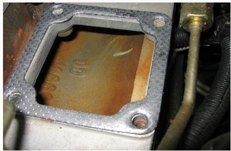
8. This kit has 2 Long Stud (J) and 2 Short Stud (H), to determine the correct stud length for your truck, thread each a long and short stud (short threaded end first) into the manifold bolt holes farthest from the valve cover. Measure the height of the stud from the heater grid block upward. Use the studs that are approximately 1.125".
