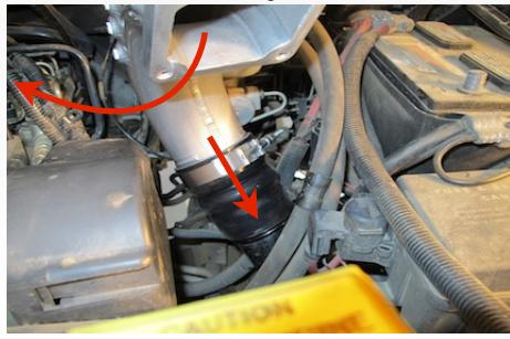
16. Install the two M8 Socket Head Screw (E) and M8 Washer (D) through the two holes. Hand tighten for now.
