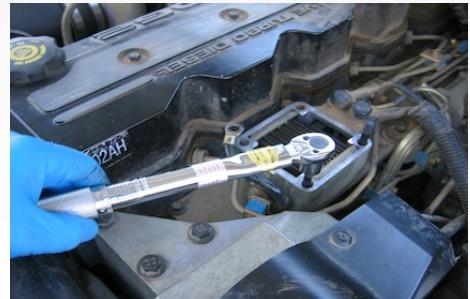
11. Apply a thread sealant such as Teflon tape to each 1/8" NPT Plug (G) and insert the plugs into the ports you will not use on the S&B elbow. Use a 3/16 hex socket and tighten, do not exceed 40 In. lbs.
