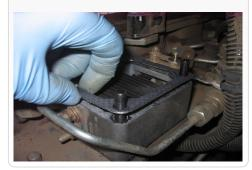
14. Remove the OE nut at the lower dip stick tube bracket and carefully push the tube back about one inch.
