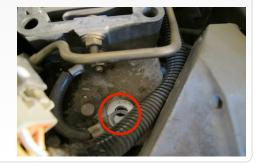
18. Slide the OE t-bolt clamp up onto the Silicone Adapter (S) and torque the clamp to 90 ln. lbs.
