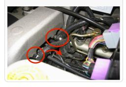
5. Remove the 4 bolts that secure the elbow to the manifold and remove the elbow from the vehicle. Careful not to let any debris fall into the manifold. Note: If the OE bolt threads were corroded and rust deposits have fallen through the bolt holes into the manifold use a vacuum to clean it out.
