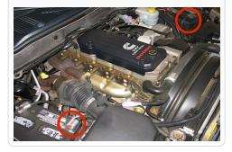
Loosen the upper hose clamp at the OE elbow and disconnect the hump hose from the elbow.
