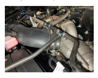
Place two #72 Hose Clamps (J) onto the ends of the Ribbed Coupler (D). Install one end of the Ribbed Coupler (D) onto the Upper Housing (E). Tighten the #72 Hose Clamp (J) on the end installed onto the Upper Housing (E).
