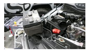
Disengage the red locking clip, press down on the tab, then pull out to disconnect the MAF sensor harness from the MAF sensor.
