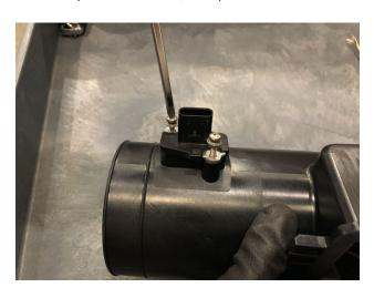
Remove the filter minder and filter minder grommet from the stock airbox and install them into the Upper Housing (E). If for some reason you do not have the stock filter minder and filter minder grommet, you can use the supplied Filter Minder Grommet (W) to seal the hole in the Upper Housing (E).
