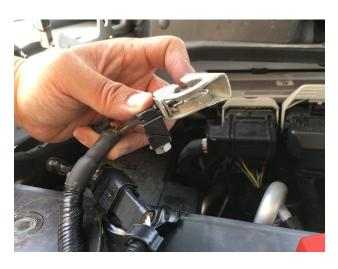
Remove the nut on the positive battery terminal and disconnect the secondary cable. Set the nut aside, it will be reused in Step 46.
