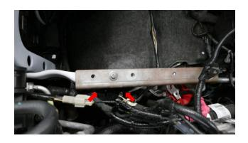
Remove the two screws securing the stock battery tray to the stock intake inlet.
