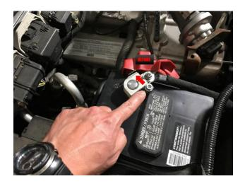
Before securing the wiring terminal to the battery post, place the red BATT wire, from the Fan Wire Harness (S), into the clamp nut assembly. Once added, place the wiring terminal onto the battery post and secure the assembly with the terminal clamp nut torqued to factory specifications, 80 lb-in (9 Nm).
