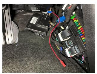
Unscrew the other end from the body of the red Posi-Lock (Y) then insert the green/orange CBP22 wire from the stock wire bundle, prepared in Step 20, through the end cap of the red Posi-Lock (Y).
