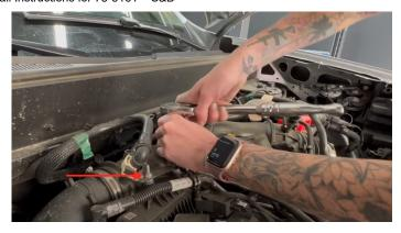
Now that you have removed the (2) nuts, you may successfully disconnect the electrical sensor and remove the retainer clips.
