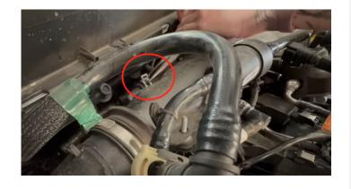
Using a Quick-Connect tool, you will need to disconnect and remove the remaining quick-connect hose. (located towards the front end of the intake tube)
