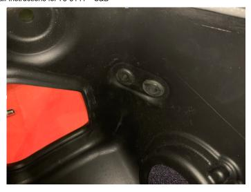
From the inside of the Air Box install Shoulder Bushings into the Grommets.
