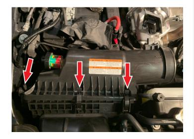
Remove the stock intake box lid and tube from the vehicle.
