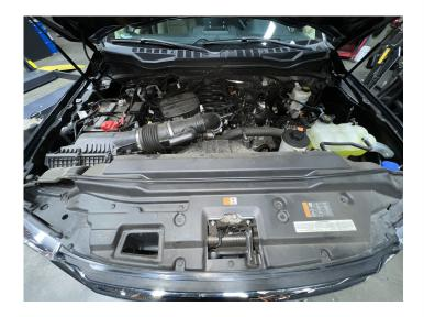
Disconnect the MAF sensor electrical harness by disengaging the white locking clip, pressing down on the tab, then pulling away from the MAF sensor.
