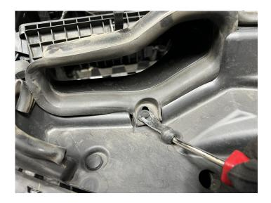
Remove the stock front inlet and box out from the vehicle.
