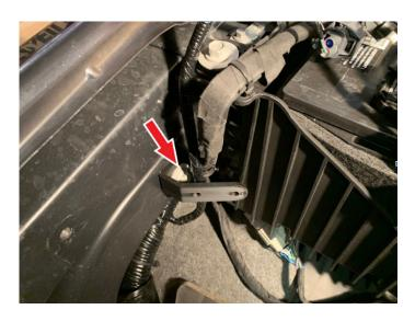
Attach the Air Box Inlet to the Air Box.
