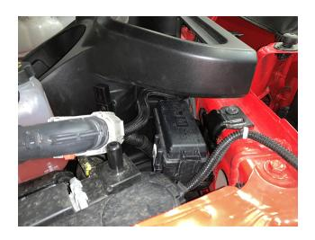
Attach the large, forward wire harness to the Harness Bracket.
