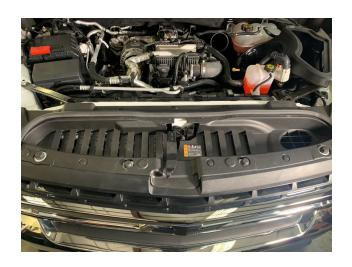
Attach the Push In Cable Tie (26) into the upper hole in the back side of the airbox, and loop it back into itself, leaving it loose. This tie will be tightened at the end of the installation.
