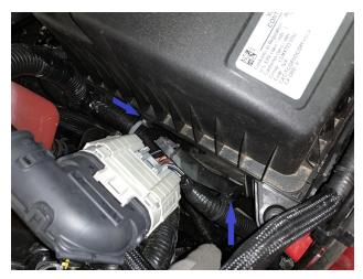
Disconnect the MAF Harness. Pull back on the red tab to unlock the connector. Press down on the black tab directly under the red tab and pull rearward to disconnect the connector.
