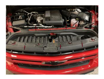
Disconnect and remove the support brace near the stock air inlet tube. Tool Needed: 13mm Wrench or Socket.
