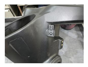
Install the Panel Grommet (16) into the Air Box Mounting Bracket (24). Install the Machined Aluminum Shoulder Washer (15) into the Panel Grommet. Install the Air Box Mounting Bracket (24) with the  $\frac{1}{4}$  x 20 Button Head Cap Screws (17). Tool Needed:  $\frac{5}{32}$  or 4mm Hex Key.
