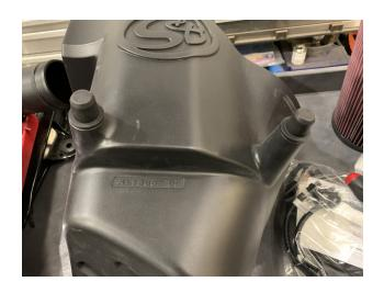
Install the Airbox into the vehicle, sliding the prongs into their holes and lowering the box onto the stud. Loosely Reinstall the nut with a captive washer onto the stud.
