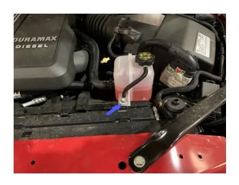
Remove the bolt holding down the fuse box bracket, and push the fuse box as far forward and out of the way as possible. Tool Needed: 10mm Wrench or Socket.
