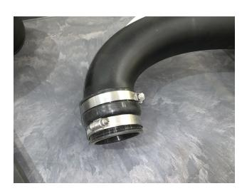
Feed the long tube through the engine bay and slide the coupler onto turbo inlet. It is possible to feel the mounting ball for the bracket, shown in the photo, and with the tube on the turbo inlet the alignment should be close. Line the ball and bracket up and push down on the tube until it seats. Tighten the hose clamp on the turbo inlet. Tool Needed: 7mm nut driver or Flat Blade Screwdriver.
