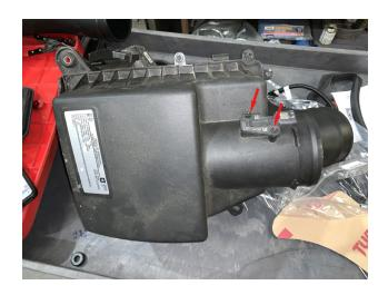
Find the Short S&B Intake Tube (2) and HP1407-00. Install the MAF Sensor into the Short S&B Intake Tube using the MAF Pad (9), MAF Gasket (10), and supplied screws (11). Take care that the MAF pad and sensor are oriented correctly on the MAF boss on the tube, as shown. Tool Needed: Philips Head Screwdriver
