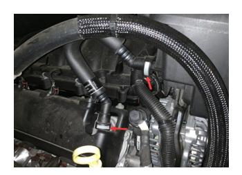
Loosen the hose clamp next to the MAF sensor and also the hose clamp on the throttle body.
