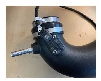
Snap-in a Push-In Cable Tie (26) into the insert on the back of the intake tube. Loop the cable tie into itself and feed the MAF Harness Extension Cable through it
