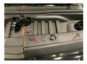
Disconnect and remove the support brace.
