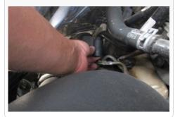
28. Slide the Hose (T) completely over the sleeve and tighten #16 Hose Clamp (Y).
