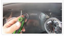
E. Install Monitoring Light (AD) into the drilled out hole, screw the locking nut onto the back of the panel by running the wire through the nut.
