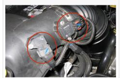
3. For the MAF sensor, slide the red locking tab up then depress the black lever while disengaging the connector. For the IAT sensor just depress the grey lever while disengaging the connector.
