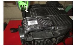
13. A good amount of force may be required to remove the motor from the factory air box. The motor shaft may need to be rotated while removing from the factory butterfly valve in the factory air box. Grab both the butterfly valve and motor and twist while pulling out.
