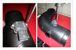
**12.** Remove the Factory Swing Gate Motor (L) from the side of the factory air box using a T-27 torx key.
