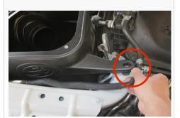
25. Push down on air box and tighten the provided Retaining Bolt (H). If the bolt does not align correctly please go back to step 36 to make sure the box is set correctly.
