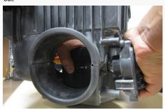
14. Mount the swing gate motor onto the bottom of the Intake Air Box (I) using Spacer (K) and #10-24 Screw (M) and #10 SS Washer (BB).
