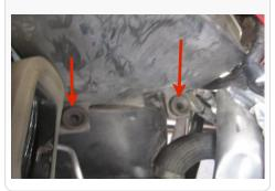
24. After dropping in the box move hose forward to let the box drop down completely. Once box is dropped flush reconnect hose clip to the vehicle.
