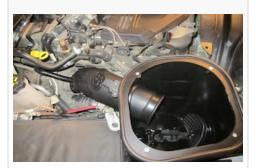
23.(a) When fitting the S&B intake box into the vehicle please make sure that the stand-off post on the bottom of the air box fit properly into the holes on the air box tray in the vehicle.
