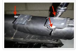
11. Place MAF sensor and IAT Sensor onto the Intake Tube (X) using the 8-32 pan Head Screw (U) and Gasket (V&W).
