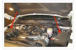
2. Disconnect the electrical connection for the Intake Air Temp (IAT) sensor and the Mass Air Flow (MAF) sensor then unsnap the wire loom from the tube.
