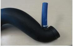
20. Install Intake Tube (X) into Air Box (I) by sliding the tube through the Tube Seal (Q). This should be a snug fit. A perfect seal is not required.
