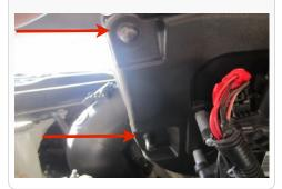
23.(b) Reach under the air box to feel if the posts pushed through the holes (grommets). Be careful not to push to hard or the tabs will break off the battery tray.
