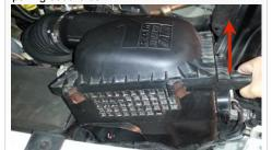
8. Disconnect the harness from the Factory Swing Gate Motor (L) that is located on the side of the factory air box. Press in the locking button on the connector and pull out.
