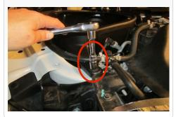
**26.** Connect Silicon Adapter (Z) to turbo and tighten #64 Hose Clamp (AA). Please make sure the coupler is push all the way onto turbo before tightening completely.
