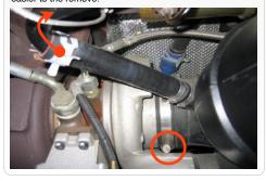
Loosen the hose clamp on the intake tube.
