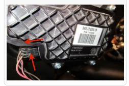
9. Once the harness is disconnected, completely remove the factory air box and intake tube by lifting up and out.
