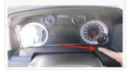
**D**. Carefully drill a hole using a 5/16" drill bit, use lower rpm speeds and start hole with smaller bits like a 1/8" or 3/16" to avoid damage to panel.
