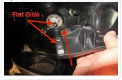
18. Do NOT remove or manually turn the Swing Gate Arm (S) after it is attached to the motor as this could damage the arm. If removal of Swing Gate Dam (N) is desired, leave the Swing Gate Arm (S) attached to the Factory Swing Gate Motor (L), and carefully unbolt the Swing Gate Dam (N) from the Swing Gate Arm (S).
