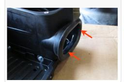
15. Install the tube seal (H) into the air
