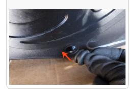
14. Install the fender seal (O) onto the air box (L).
