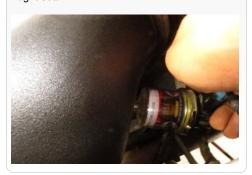
**33.** Reconnect all battery cables, positive cables first. Inspect your installation, make sure the kit is properly positioned and all fasteners are secure. The installation is now complete.
