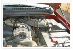
2. Remove the OE battery cover by pressing in both tabs on the front of the battery.
