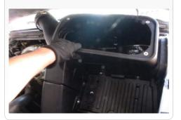
22. Install the provided bolts (S) and washers (N) through the battery tray which should thread through to the factory clip nuts on the bottom.
