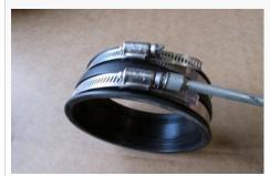
19. Slide the coupler with both hose clamps onto and over the intake tube. Push the coupler past both stop beads leaving the end of the tube exposed.
