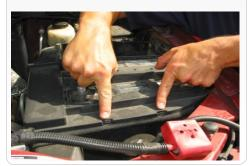
3. Remove the battery bolt and wedge then remove the battery from the vehicle.
