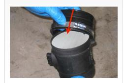
13. Connect the MAF sensor assembly to the S&B Filter Adapter ( I ) and secure using a #60 Hose Clamp (J).
