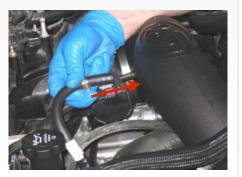
18. Place the S&B Air Filter (D) into the S&B Air Box (G), rotate the filter about a 1/4 turn for clearance and slide onto the flange and secure the # 80 Hose Clamp (E).
