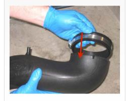
16. Place another # 60 hose clamp (J) on the Hump Adapter (L) then insert the small end of the S&B Tube (M) into the S&B Hump Adapter. Then position the other end of the tube over the throttle body and firmly secure the # 72 Hose Clamp (N), then secure the # 60 Hose Clamp (J) at the Hump Adapter.
