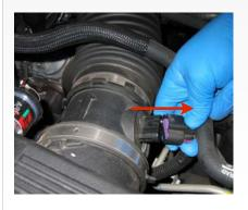
4. Pull the crankcase vent line from the OE intake tube and then from the engine along with the rubber connector and remove it from the vehicle.
