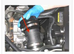
$15. \ \, \text{Slide the S\&B Throttle Body Adapter (O)} \\ \text{over the S\&B Tube (M) along with the \# 72} \\ \text{Hose Clamp (N), do not tighten at this step.} \\$
