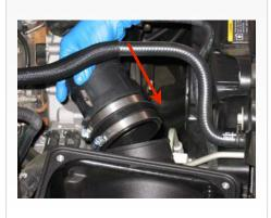
14. Slide the S&B Hump Adapter (L) over the MAF sensor's flange and secure using a # 60 Hose Clamp (J).
