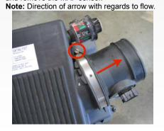
$9. \ \mathsf{Remove} \ \mathsf{the} \ \mathsf{OE} \ \mathsf{air} \ \mathsf{box} \ \mathsf{tray} \ \mathsf{from} \ \mathsf{the}$ vehicle. Four of these bolts if long enough, may be used to secure the S&B air box to the vehicle. If not use the supplied M6 allen head
