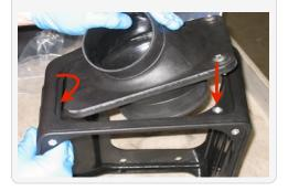
11. Place the air box assembly into the vehicle, align the four holes with the OE mounting locations and secure using either the OE bolts or the supplied allen head screws and SS washers.
