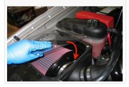
21. Reconnect the MAF sensor electrical connection.
