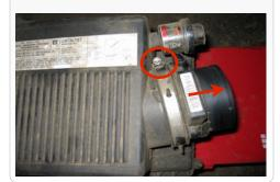
9. Remove the OE tray from the vehicle. Four of these bolts (if long enough), can be used to secure the S&B air box to the vehicle. If too short, then use the supplied allen head screws an SS washers.
