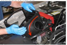
12. Slide the Straight Adapter (F) over the MAF sensor's metal flange, secure using a #60 Hose Clamp (J).
