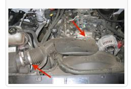
7. Pull the OE air box towards the engine and up to release it from the vehicle.
