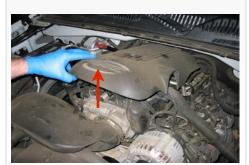
3. Disconnect the electrical connection to the MAF sensor at the OE air box.
