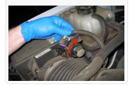
If equipped: Pull the crankcase vent line from the OE intake tube and then from the engine along with the rubber connector and remove it from the vehicle.
