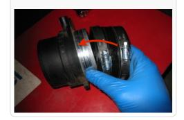
13. Connect the MAF sensor assembly to the Filter Adapter (I) and secure using a #60 Hose Clamp (J).
