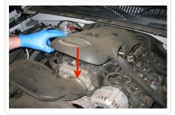
23. Reconnect both batteries. Inspect your installation, make sure the kit is properly positioned and all fasteners are secure. Affix the CARB sticker near the intake kit. The installation is now complete.
