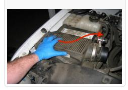
8. Loosen the hose clamp on the OE air box and remove the MAF sensor. Note: The direction of the air flow through the sensor.
