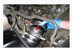
15. Slide the Throttle Body Adapter (O) over the Intake Tube (M) along with the #72 Hose Clamp (N), do not fully tighten at this time.
