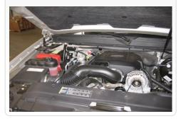
If equipped: Loosen the retaining bolt and pull up and out to remove the engine cover from the vehicle.
