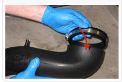
16. Place another #60 Hose clamp (J) on the Hump Adapter (L) then insert the small end of the Intake Tube (M) into the Hump Adapter. Then position the other end of the tube over the throttle body and firmly secure the #72 Hose Clamp (N), then secure the #60 Hose Clamp (J) at the hump adapter.
