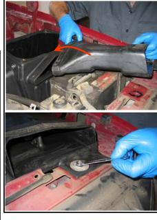
**19.** Install the S&B air filter (C) to the S&B air box adapter (H), secure the # 72 hose clamp.
