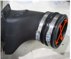
**13.** Attach the S&B air box adapter (H) to the S&B air box (F), latch the bottom and use the 5/16 screws (G) to secure the top.
