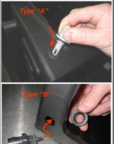
**11.** Install 2 S&B Grommets (K) into the bottom of the S&B air box (F)
