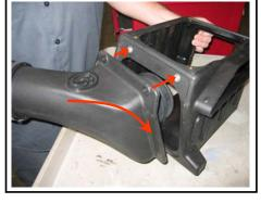
Place the S&B air box assembly in the vehicle. Before seating the grommets, reconnect the temp. sensor electrical connecto
