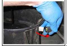
8. Pull up and push towards the firewall to release the OE air box from the rubber grommets, remove it and the grommets from the vehicle.
