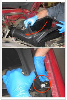
**15.** When the S&B air box is in place, secure using the OE nut and washer.
