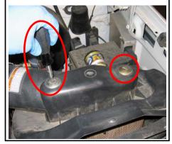
assembly, then remove the OE air filter.
