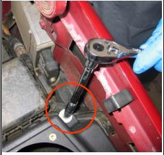
**16.** Center the S&B hump adapter (J) over the gap between the tubes. Secure both # 64 hose clamps (I).
