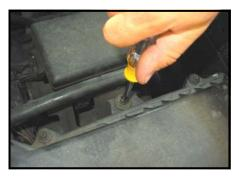
4. Remove vent hose from air box and valve cover.
