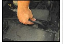
Install adapter assembly to filter.
