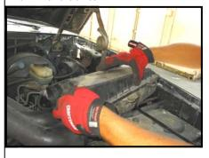
6. Install the "L" bracket to the end of the filter as shown
