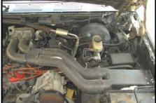
2. Unclamp intake hoses from the air box. 5 Remove air box.
