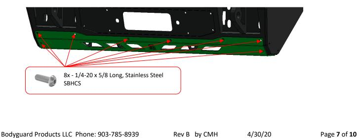
Next install the skid plate bracket to the crossmember by inserting a teardrop bolt into the frame.
