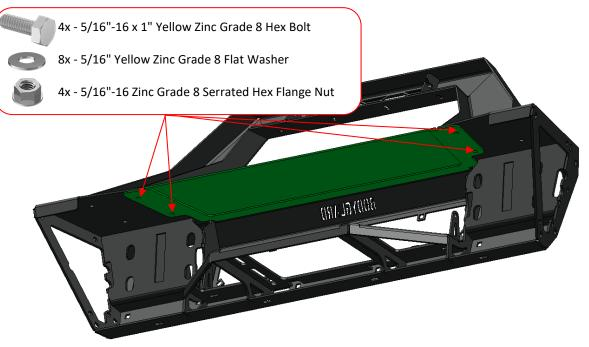
2. Install the light bar tabs onto the bumper. Then install your 20" double row light bar to these tabs
