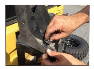
2. Place Brake light extension on rear tire mount with triangle cutout facing front of vehicle.
