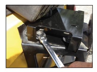
4. Attach brake light tower to brake light extension with supplied hardware.
