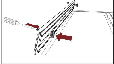
Set the cover (A) in the folded position on the side rails (B & C) towards the cab of the truck. Confirm the cover is evenly spaced between the rails.
