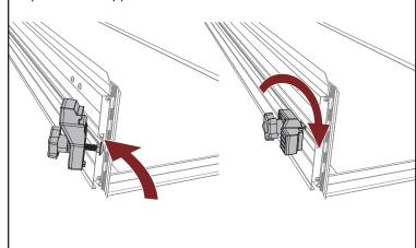
Position the buckle ends (I) with the open side facing the bed cover panel. Use a screwdriver to install the two buckles into the pre-drilled holes on the front header panel with the provided screws (J). **DO NOT use a screw gun, securely tighten by hand only.**
