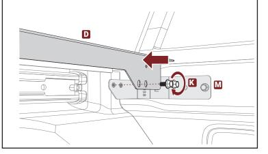
Install the adaptor rail driver side (D) by lining up the studs with the holes in the rear bracket using two M6 flange mounting bolts (K) and two 1/4-20 nuts (L). Repeat on the opposite side using the passenger side adaptor rail (E). Now tighten, using a 7/16" socket in front and rear on both sides.
