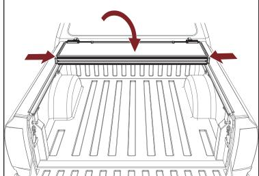
Confirm the retainer clamps (G) are positioned around the side rails (B & C) correctly as shown below. Tighten the retainer clamps by turning them clockwise until the lock washer is secure.
