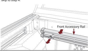
Installing Front Mounting Brackets: Use the driver side front mounting bracket (M) labeled with the letter "L". Locate the pre-bent tab on the front bracket and place in the upward most hole located towards the front corner of the bulkhead on both sides. Repeat on passenger side using the passenger side front mounting bracket (N) labeled with the letter "R".
