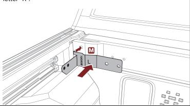
If you do not have a front accessory rail, as mentioned in step 2, proceed to install one M6 flange mounting bolt (K) into the front bracket (M) in the second slotted hole to the right as shown. Repeat on the passenger side using the passenger side front mounting bracket (N) labeled with the letter "R".
