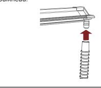
Before placing the cover (A) onto the vehicle, slide two front cover retainer clamps (G) into the track on the underside of the cover (A) near the cab. Confirm the cover retainer clamps fit properly into the cover rail for optimum fit. Repeat on the opposite side of the cover.
