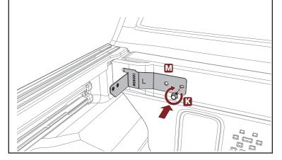
If you **DID** remove the front accessory rail, as mentioned in step 2, proceed to install the accessory rail over the front bracket (M) you just installed aligning the holes in both using one M6 flange mounting bolt (K) through both and into the bulkhead. Repeat on passenger side using the passenger side front mounting bracket (N) labeled with the letter "R". Then tighten bolts.
