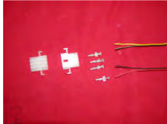
Figure 6. These are the plug assemblies. The male end is used on the mirror. The female end is used on the vehicle harness.
