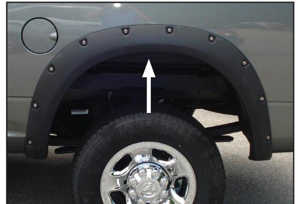
9. Hold flare to vehicle and start supplied Phillips screws and factory bolts into existing holes and holes covered in plastic tabs and clips. *Do not tighten.* Press firmly on flare and tighten all screws. Complete rear flare installation.
