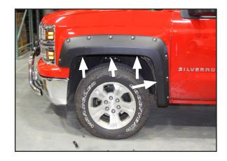
11. Remove factory rear mud guards. Using T-15 Torx bit, remove 4 factory screws from lower front of rear wheel well.
