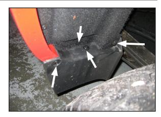
12. Remove plastic mud guard and re-install the 2 screws indicated in the diagram.
