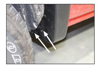
6. Holding flare firmly against the vehicle, mark the hole location of the forward most hole in the flare.
