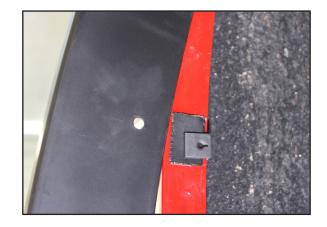
18. To complete installation, use supplied edge trim tool to seat edge trim against vehicle with curved end; slide it under trim along vehicle fender. Use flat end of tool to seat trim against flare; slide tool between trim and flare.
