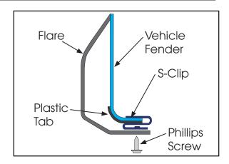
9. Return flare to proper position, and install #10 x 5/16 phillips screw through flare into S-clip.
