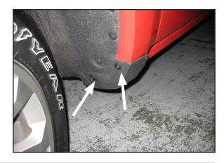
5. Firmly hold flare to vehicle. Reuse the 2 existing mounting holes and the supplied #8 x 3/4 phillips screws to fasten the rear portion of the flare.
