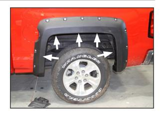
17. As with front flares, install S-Clip over inner lip edge of fender centered over plastic tabs. Install flare using supplied #10 x 5/16 Phillips Screws into S-Clips. Moderate pressure against the flare may be needed for mounting holes to align. Repeat steps 11-17 for opposite side.
