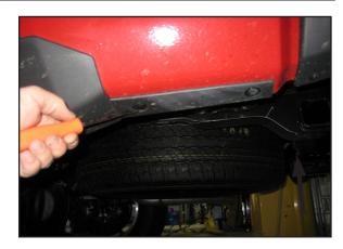
14. Firmly hold rear flare to fender and install supplied #8 x 3/4 Phillips head screws through two lower-most holes in flare into existing mounting holes in fender.
