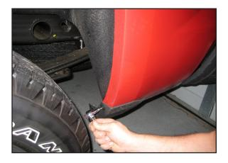
14. Using trim removal tool, remove the 2 plastic rivets on underside of vehicle, behind rear wheel well. Remove mud guard.
