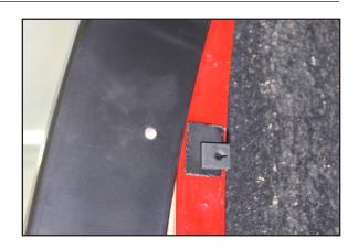
8. Refer to diagram; For proper installation of S-Clips, install S-Clip over inner lip edge of fender centered over plastic tab. Install flare using supplied #10 x 5/16 Phillips Screw. Insert through the hole in the flare and screw into S-Clip until tight. Moderate pressure against the flare, and minor adjustments of S-Clip position may be required for mounting holes to align.
