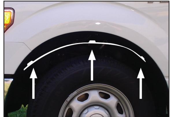
6. Hold flare to fender and install factory screw into factory hole toward rear of wheel well using 7/32" socket. Continue to hold flare and drill through bumper cover with a 1/4" drill bit using forward most hole in flare as a guide.
