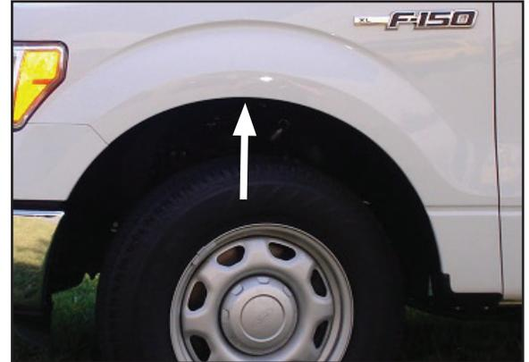
5. Install Front Flare Inner Piece using a supplied Phillips screw through installed Small Screw U-Clamp. Use factory screws and 7/32" socket to attach inner piece to factory holes.
