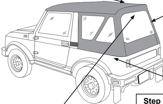
**Step Eight:** Snap the snaps on the bottom of the side panels from front to back.
