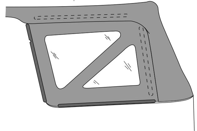
Fit the notch in plastic strip around stop in retainer
