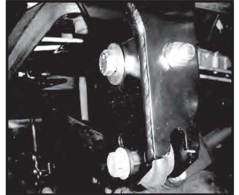
Step 4. Temporarily install the frame brace bar into the passenger side L-bracket. Adjust the length of the bar so that the L-bracket fits flush against the frame rail.
