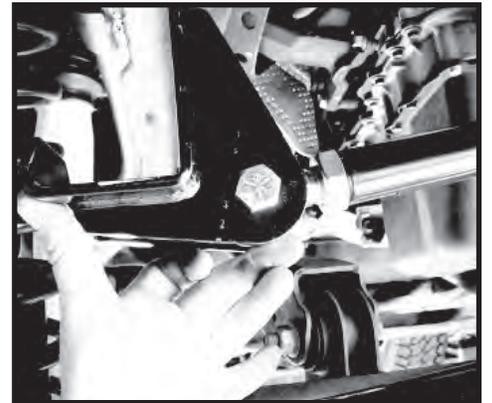
Step 5. Once you have made the adjustments to the bar and bracket, verify that the bar is perpendicular to the frame. Using a marker or scribe trace the outline of the bracket onto the frame. Mark a reference line on the bracket and frame to align after grinding.
