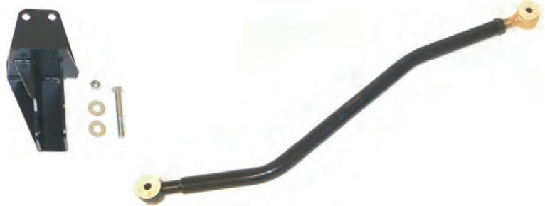
1. Please read instructions fully prior to installing the Adjustable Trac-Bar. The Trac-Bar's function is to properly locate the front axle under the Jeep body. This kit is designed to help correct this misalignment that can develop with lifts as little as 2" and up to 6". Not all lifts are the same and all final adjustments will be different for every vehicle.
