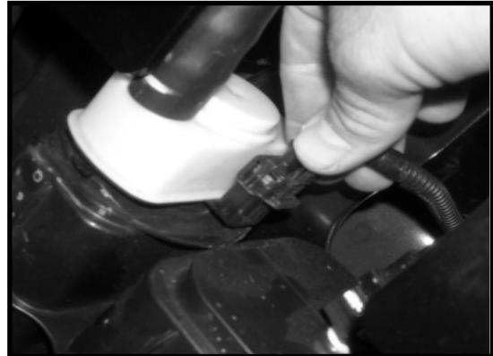
2. Remove the 3 bolts securing the vapor canister to the frame rails. 1 bolt is located at the rear of the canister and 2 are located at the front. When these bolts are removed, the canister will be suspended from the vehicle by hoses only so be sure not to let it hang.
