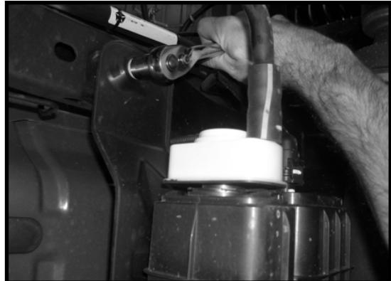
3. Slide Rear Bracket over the rear of the vapor canister toward the front of the vehicle being sure to keep the canister from hanging. It might be easier to have a partner hold the canister while sliding on the bracket.
