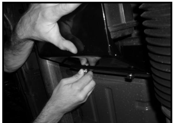
6. Tighten all bolts securing brackets to frame rails. For the bolts attaching the Front Bracket to the frame rail, use a wrench rather than a ratchet for easier access. Make sure there is no interference with any components of the driveline or exhaust before operating the vehicle.
