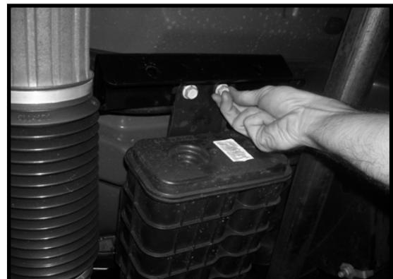
5. Fasten Skid Plate to brackets installed in steps 4 and 5. Adjust brackets and vapor canister if necessary to line up holes. Push Skid Plate up as far as it will go when tightening.
