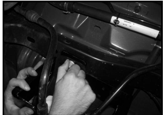
5. Install Front Bracket by replacing bolts removed in step 2. Do not tighten as assembly will have to be adjusted when skid plate is installed.
