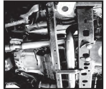
Step 2. With the factory skid plates removed, begin mounting the new transfer case skid plate. Using (3) of the supplied M12 x 35mm hex bolts and M12 washers, fasten the skid plate to the vehicle cross member. Leave these bolts loose at this time.
