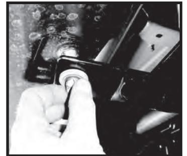
Step 4. Using the M12 x 60mm hex bolt and washers install the skid plate to the driver side of the frame. Once all of the bolts have been started tighten all of the bolts to 55 ft•lbs. Replace any skid plates that have been removed and tighten to factory specifications.
