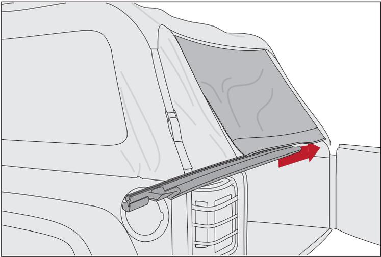
25. Install metal hook on end of rear straps into body tub through cutout in rear panel and tighten. Repeat for opposite side.
