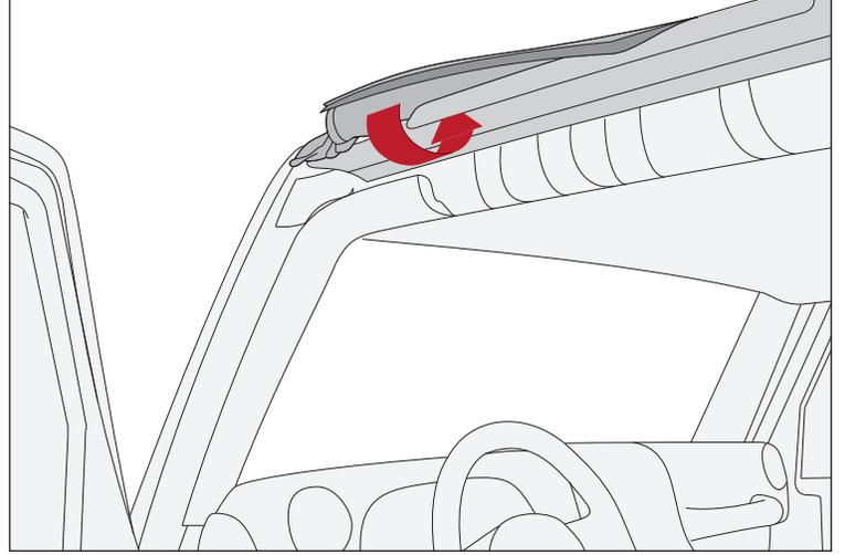
9. Pull two center straps on inside of vehicle around sport bar.
