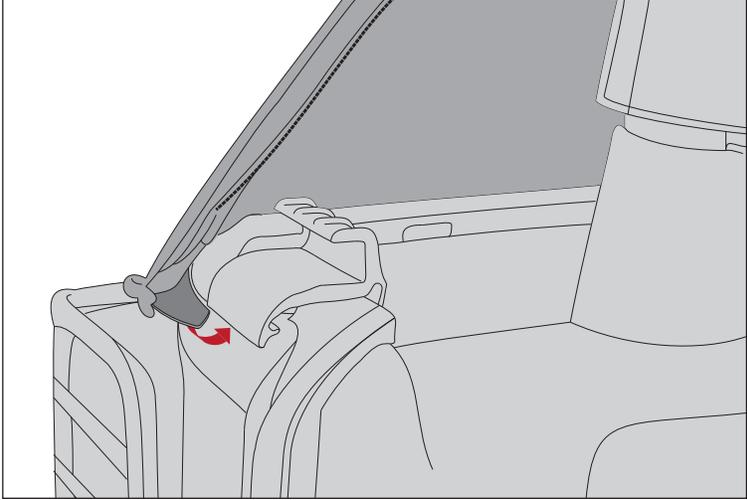
24. Slide tailgate bar into bottom of rear window and attach to receiver on tailgate.
