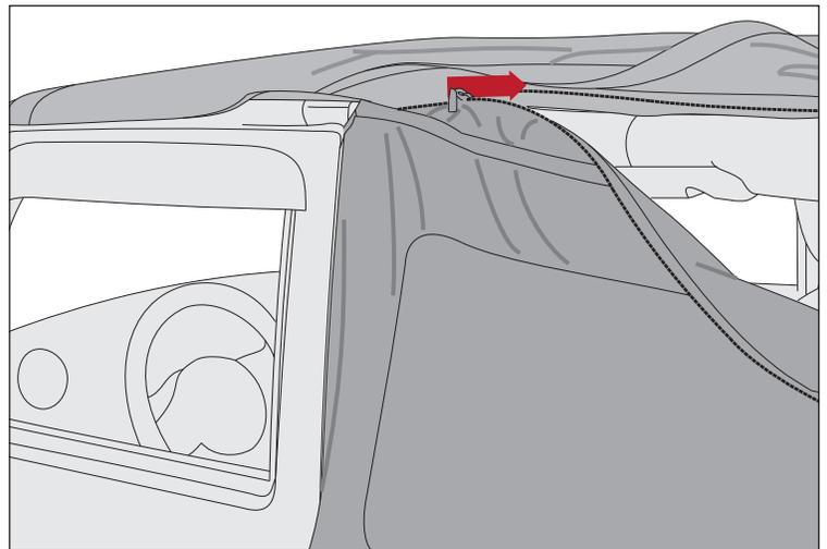
19. Pull bottom plastic retainer of side window into side groove of body tub. Repeat step 17 - 19 for opposite side.
