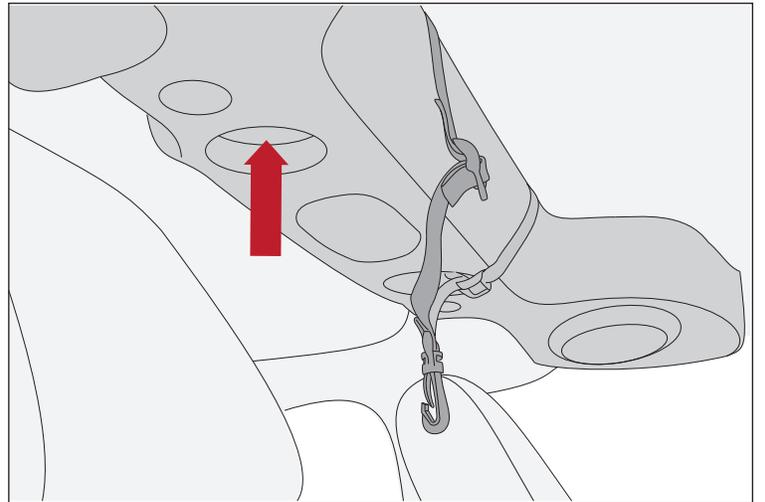
11. Loop rear side strap around rear sport bar, moving toward outside of vehicle.
