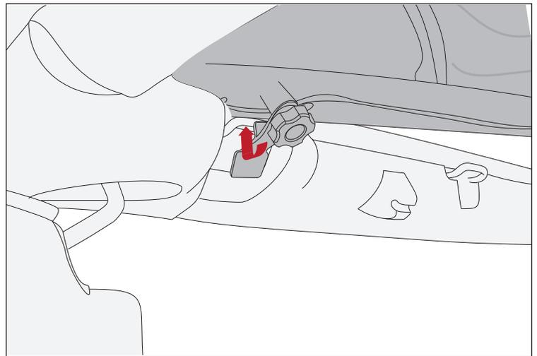
6. Attach header tab to footman loop near windshield. Ensure assembly is centered on vehicle and J-hook is placed behind and through footman loop.
