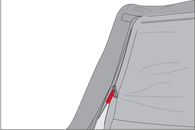
21. Loop top corner strap through plastic holder at rear corner of vehicle. Tighten strap and repeat for opposite side.
